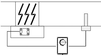
The output is rated at 20 mA max at 8 VDC.
