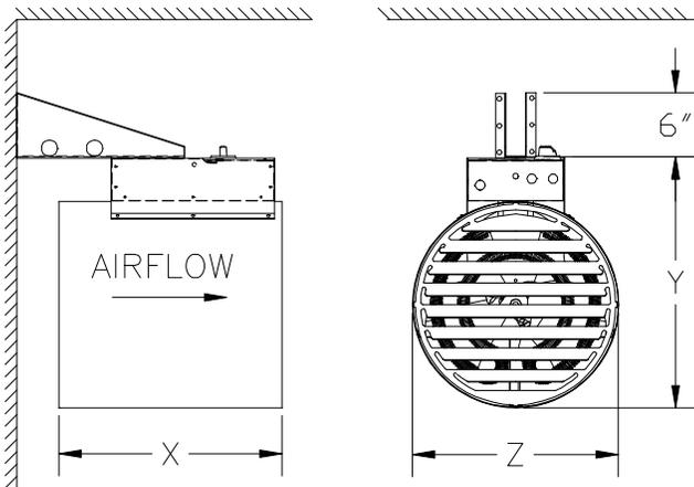
Select a location for installation such that the outlet air is not directed at an adjacent wall. Louvered discharge grills may be manually adjusted to a straighter throw with a downward pitch of less than 45°. Do not close louvers more than 45°.
